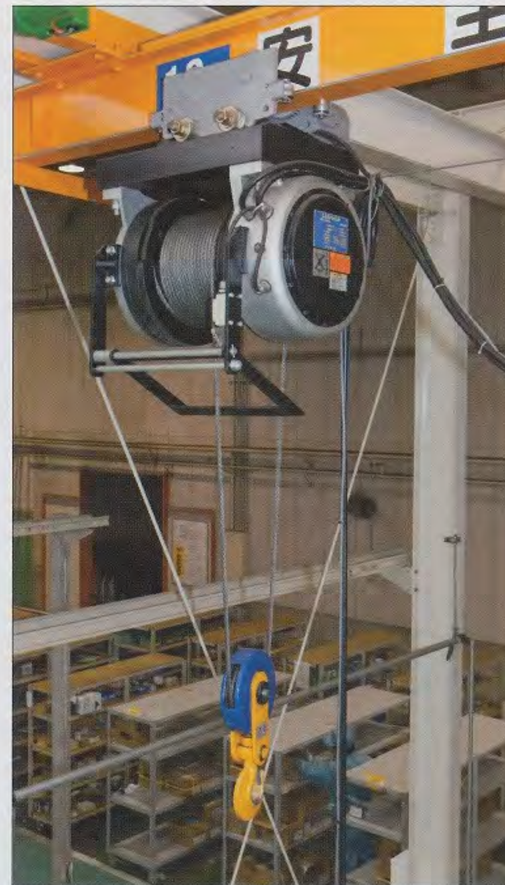
■ The electric winches can be used as hoists together with the electric trolley, gear trolley, and plane trolley. Please note that Construction Code for Cranes will be applied depending on the type of usage.
