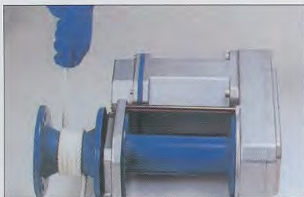
■ For pulling out cables, one-bracket-capstan drum is convenient.
