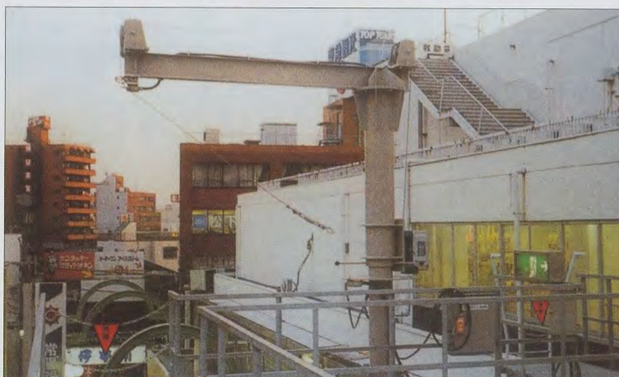
Set to a jib crane for lifting a extinguishing fire equipment
